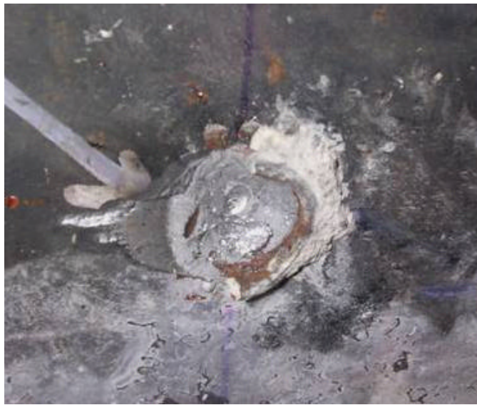
Figure B.3: Failed Specimen CIPST10: a) concrete block, b) steel plate
