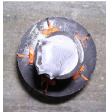
Figure 5.13: Side and top view of the failed connector (Specimen DBLNB-ST)
