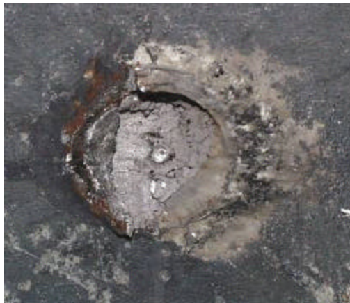
Figure B.4: Failed Specimen POSST20a: a) concrete block, b) steel plate
