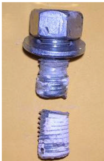
Figure 5.42: HAS-E anchor failed at two locations (Specimen HASAA40)
