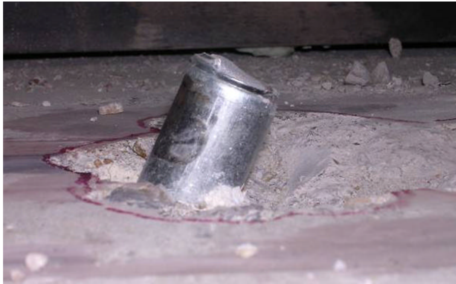
Figure 5.50: Failed Specimen HTFGB2
