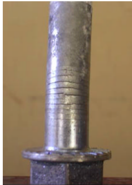
Figure 5.25 Side and front view of failed connector (Specimen WEDGB-ST)
