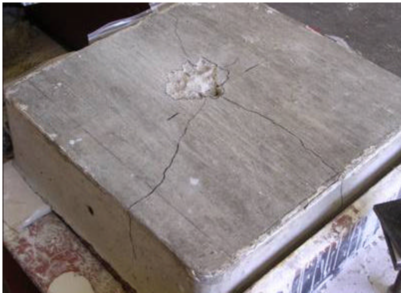
Figure 5.18: Shear failure of connector accompanied by cracking of the concrete block (Specimen HTFGB-ST)
