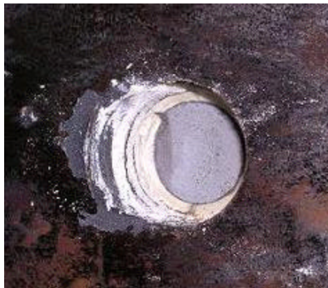
Figure 5.41: Failed Specimen HASAA40: a) concrete block, b) steel plate
