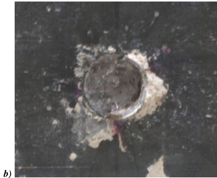
Figure D.1: Failed Specimen CIPST1: a) concrete block, b) steel plate
