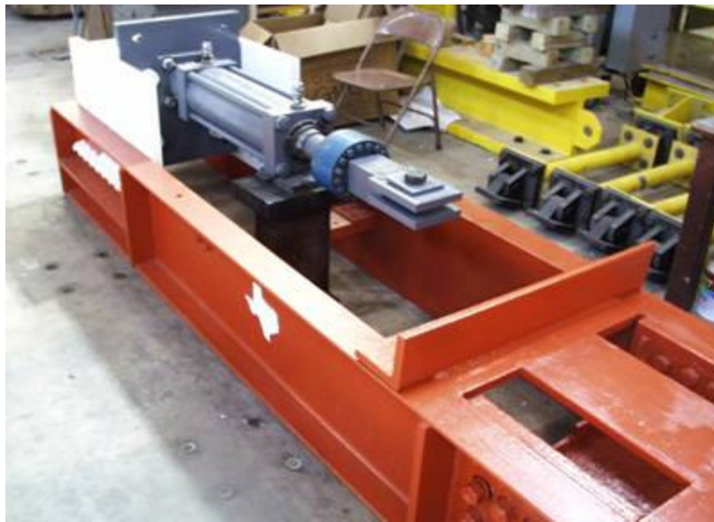
Figure 4.3: Direct shear test assembly (with bulkhead)
