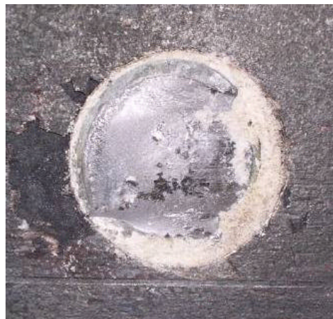
Figure 5.21: Failed HAS-E Anchor in steel plate (Specimen HASAA-ST)
