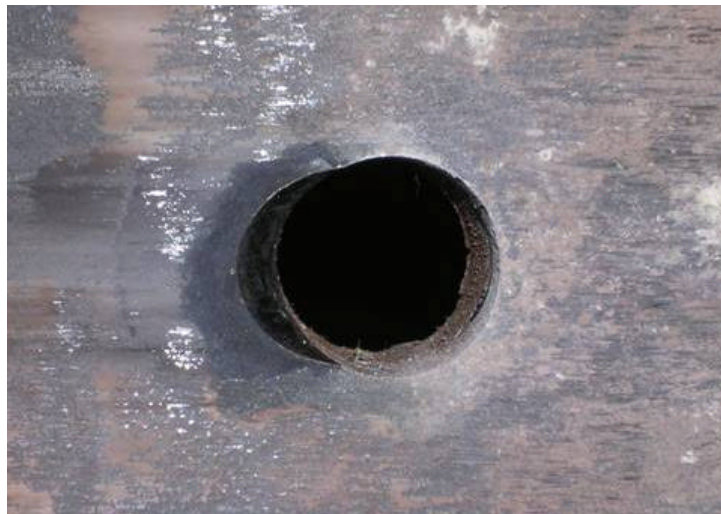
Figure 5.51: Bearing deformation of steel plate (Specimen HTFGB2)
