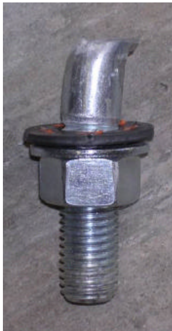
Figure 5.17: Failed connector (Specimen HTFGB-ST)
