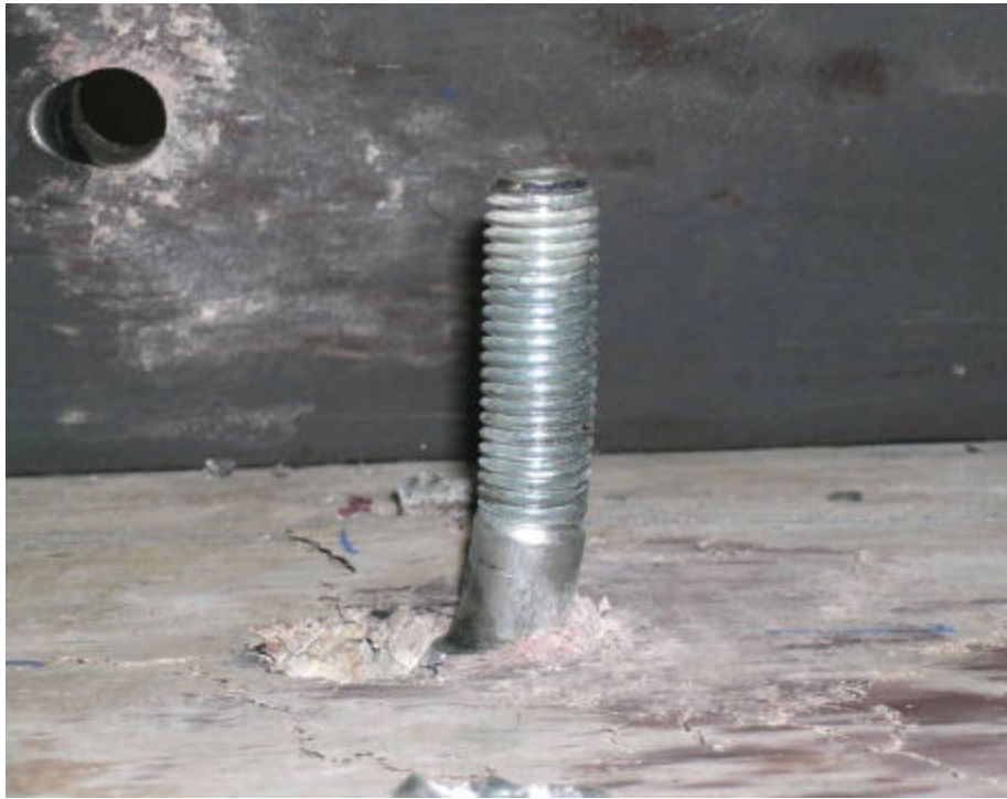
Figure D.6: Failed Specimen HTFGB3
