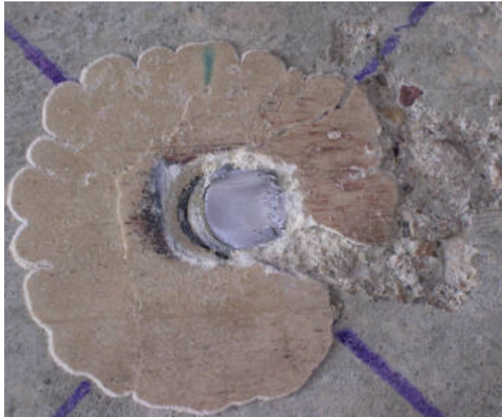
Figure 5.20: Shear failure of Specimen HASAA-ST at steel-concrete interface
