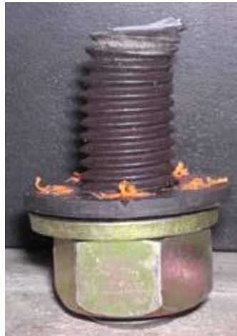
Figure 5.13: Side and top view of the failed connector (Specimen DBLNB-ST)
