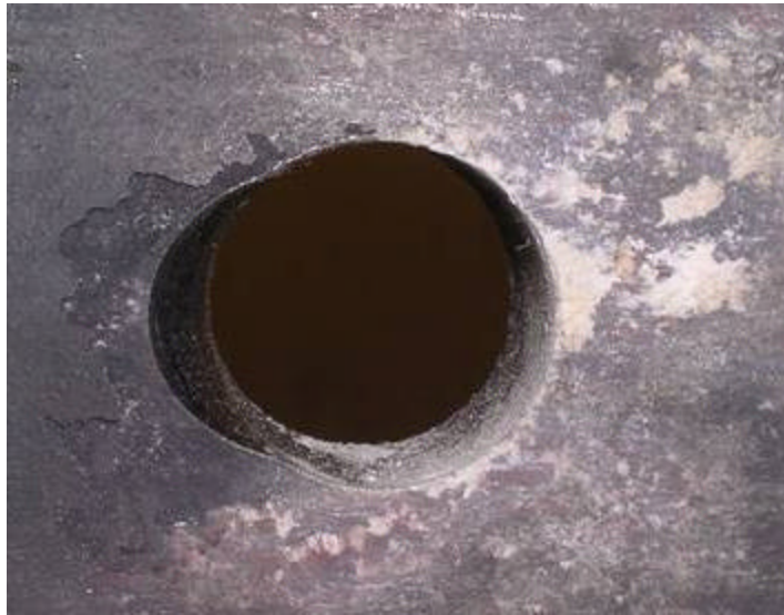
Figure 5.26 Bearing deformation of steel plate (Specimen WEDGB-ST)
