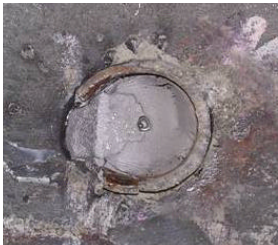
Figure 5.33: Failed Specimen POSST25: a) concrete block, b) steel plate
