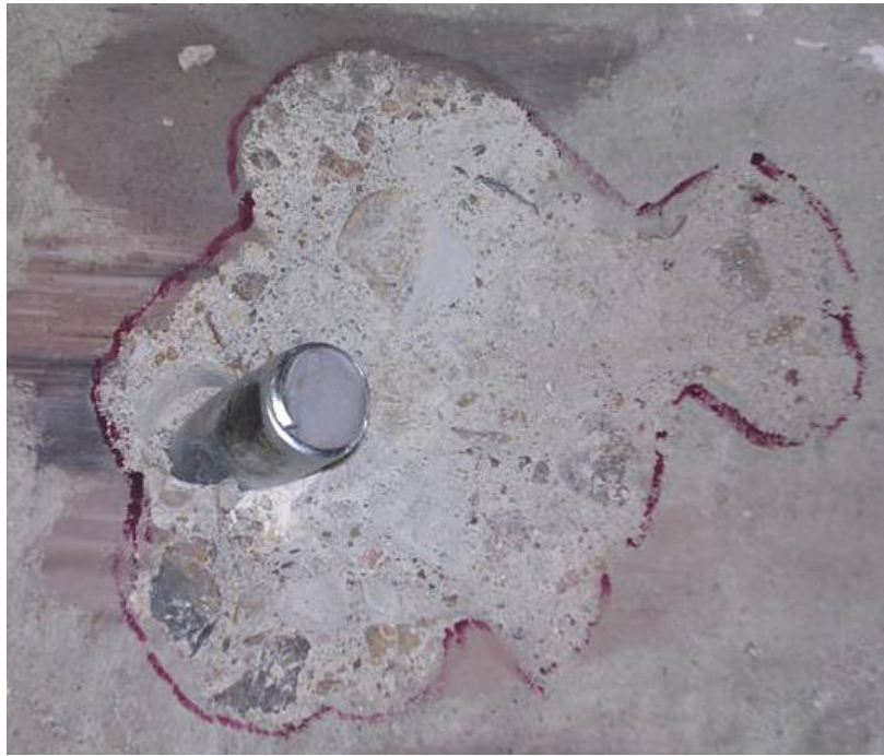
Figure D.5: Failed Specimen HTFGB2
