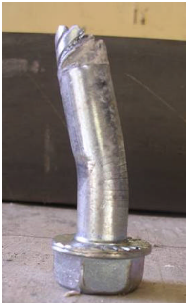
Figure 5.25 Side and front view of failed connector (Specimen WEDGB-ST)
